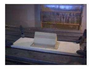
After the tool is cut it is mounted to a vacuum box or plenum. The vacuum holes are added in specific area that the plastic sheet must close in around.
